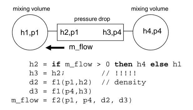
Note: Even for the most simplest case (volume – pressure drop – volume), a <u>nasty</u> <u>non-linear equation system</u> appears, since m\_flow = f2(..., m\_flow > 0); Can sometimes be fixed by replacing "m\_flow > 0" with "p4 – p1 > 0" Additionally, <u>every pressure drop</u> component is **not differentiable** at  $m_{flow} = 0$ . If non-linear equation systems occur, then this system is not differentiable at a critical point, and then every non-linear solver has difficulties.
