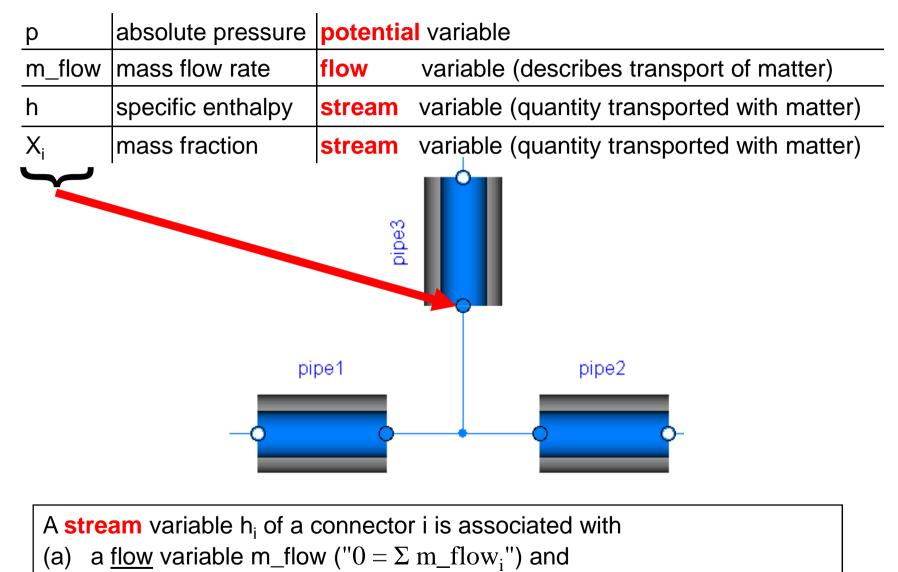
(b) a <u>stream balance</u> equation (" $0 = \Sigma m_{flow_i} < \underline{upstream}$  value of  $h_i >$ ")
