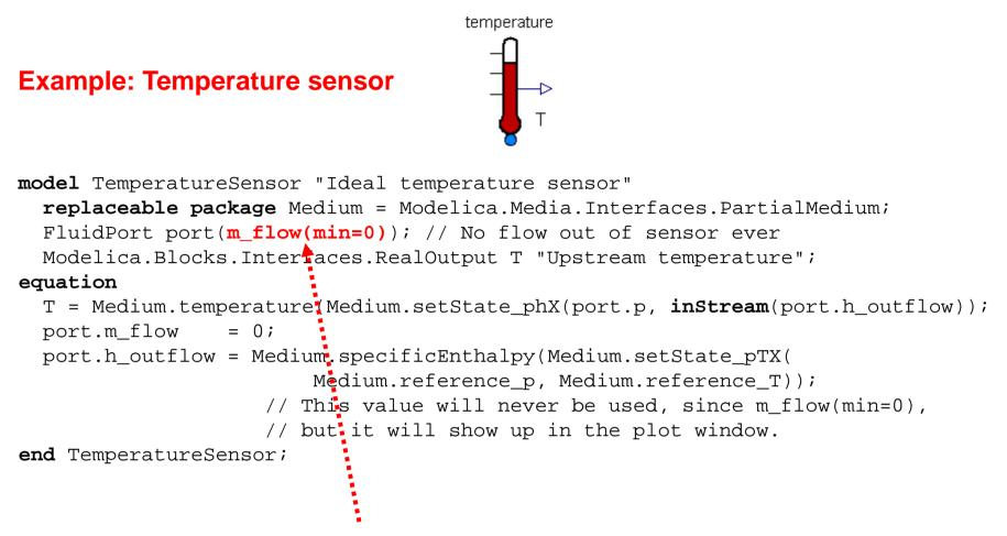
Setting "m\_flow.min=0" is very important, in order that the temperature sensor has no influence on the stream that it measures, if <u>all mass flow rates are zero</u>; since then "**max**(-port.m\_flow, $\epsilon$ ) = 0" in the **inStream**(..)-operators of the connected ports!!!
