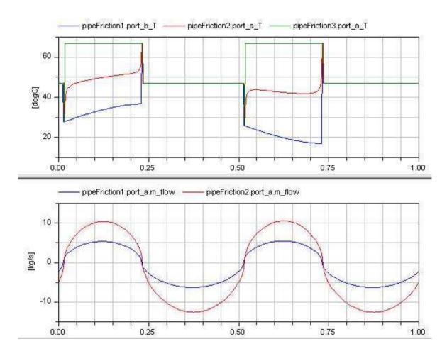
T as iteration variable (<u>discontinuous</u>) -> at m\_flow = 0, jump in iteration variable; every non-linear solver has difficulties with this.
