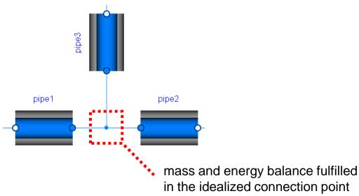
Examples of an interface for fluid components
