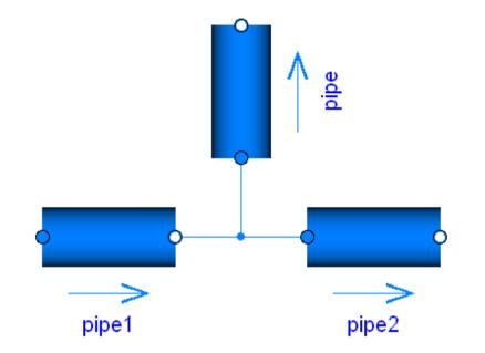
(Note: with a volume in the connection point there would be  $2+6=\frac{8}{2}$  state variables, i.e., an implicit DAE solver would have 8 iteration variables).
